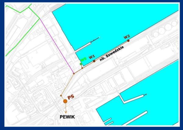
W1–W2 inlet for discharging sewage from ships including measurement of quality of sewage
